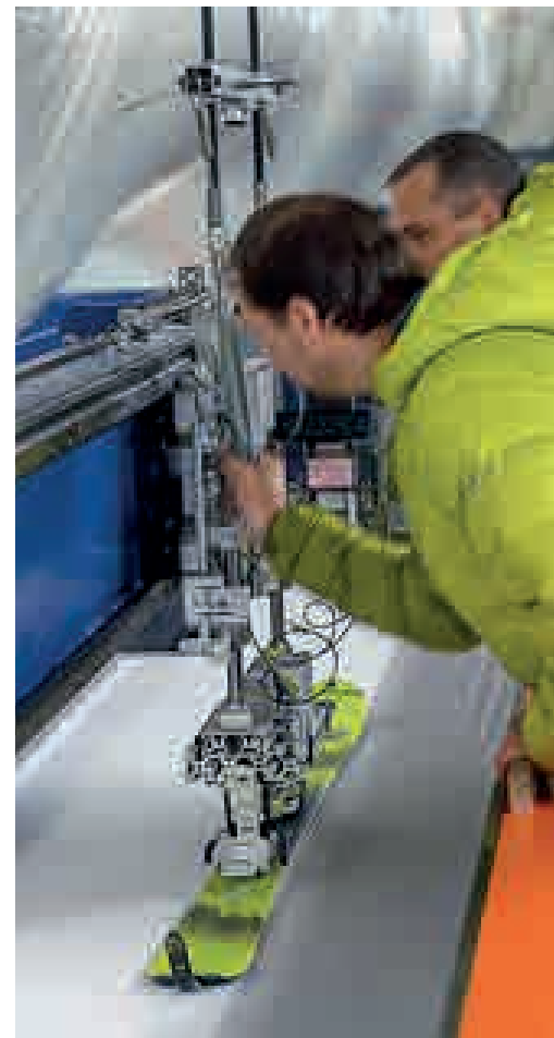
Laboratory tests on the tribometer. One of the test skins is fixed on the standard ski.
